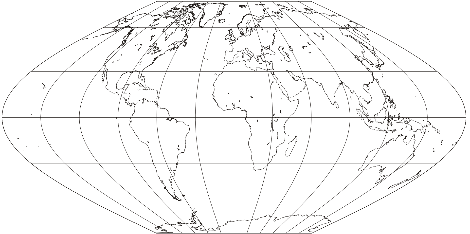
McBryde and Thomas No. 3; (Flat-polar Sinusoidal); Pseudocylindrical; Equal-area; Felix Webster McBryde and Paul D. Thomas; 1949
