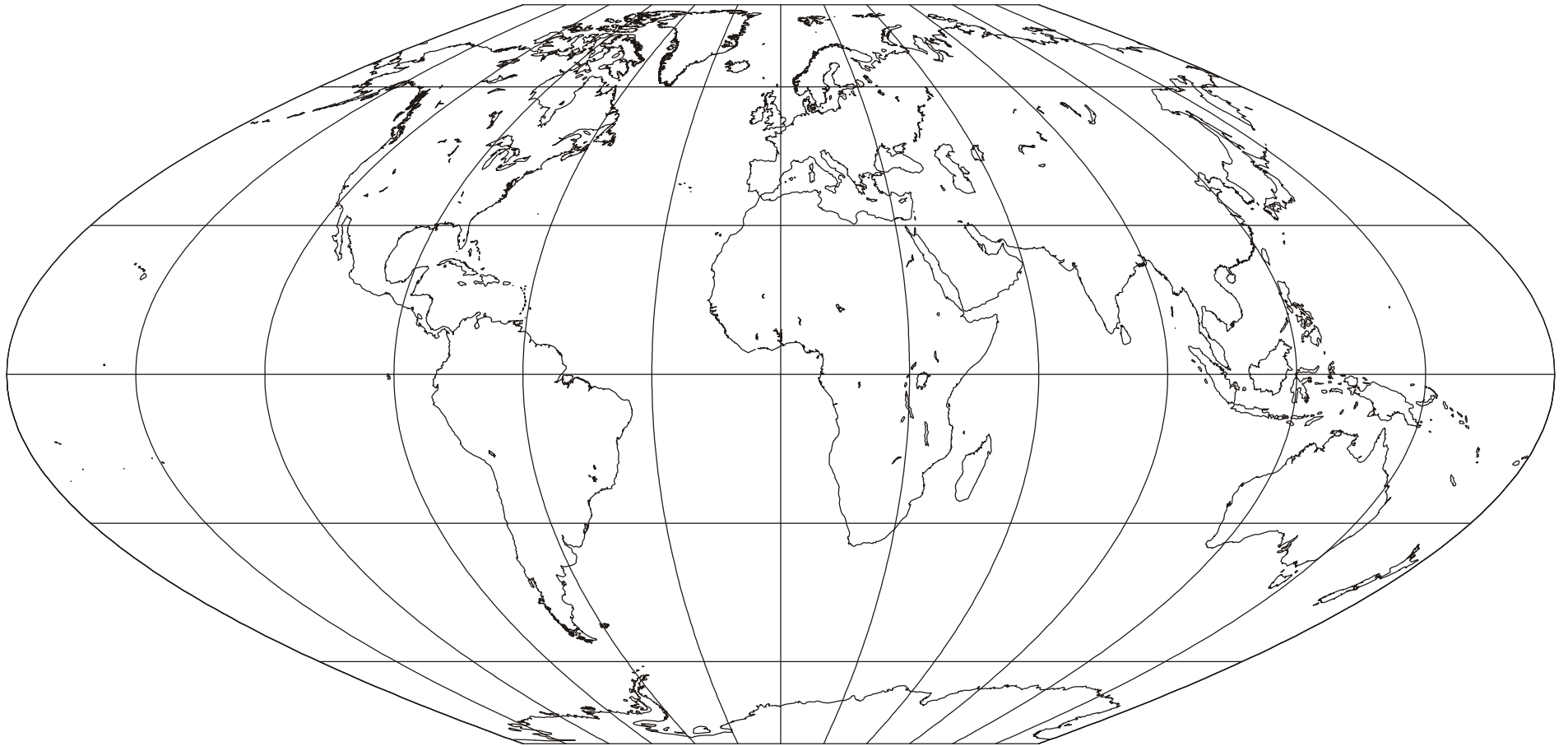
McBryde and Thomas No. 5; (Flat-polar Parabolic; Pseudocylindrical; Equal-area; Felix Webster McBryde and Paul D. Thomas; 1949
