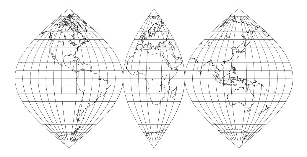
Interrupted Sinusoidal projection; Pseudocylindrical; Equal-area; As used by USGS; Source: MicroCAM software
